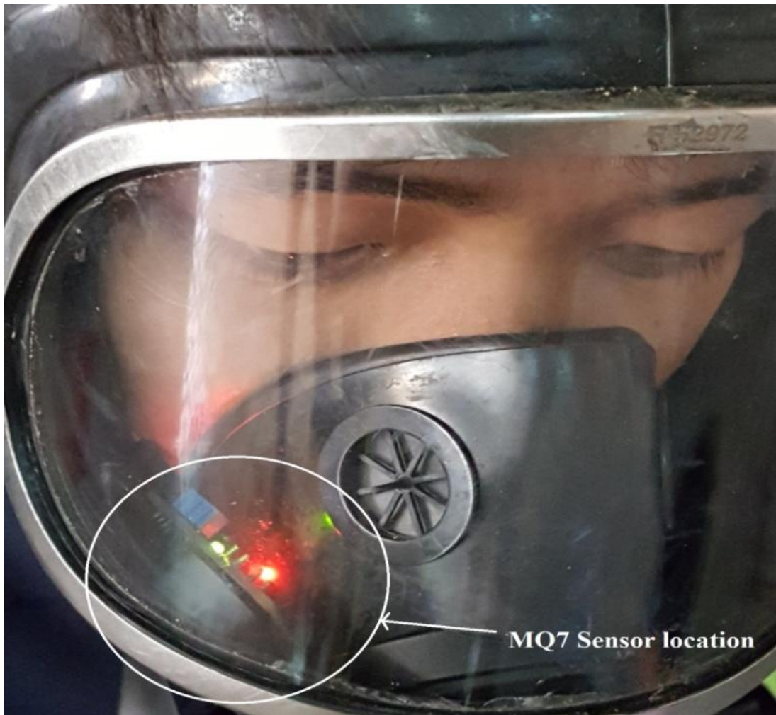
Figure 3-11– CO sensor location
