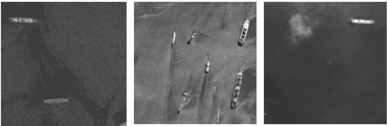
Figure 1.3. Appearance of ships in image with complex background. Strong textures sea surface and cloud can strongly affect the ship detection performance.
