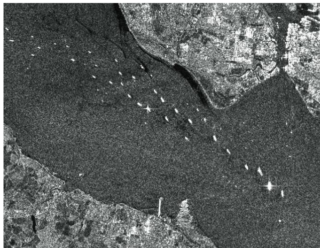
Figure 1.1. Appearance of ships in Synthetic Aperture Radar image captured by Sentinel (Source: ESA)
